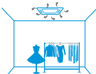
Air distribution with a dusty filter
